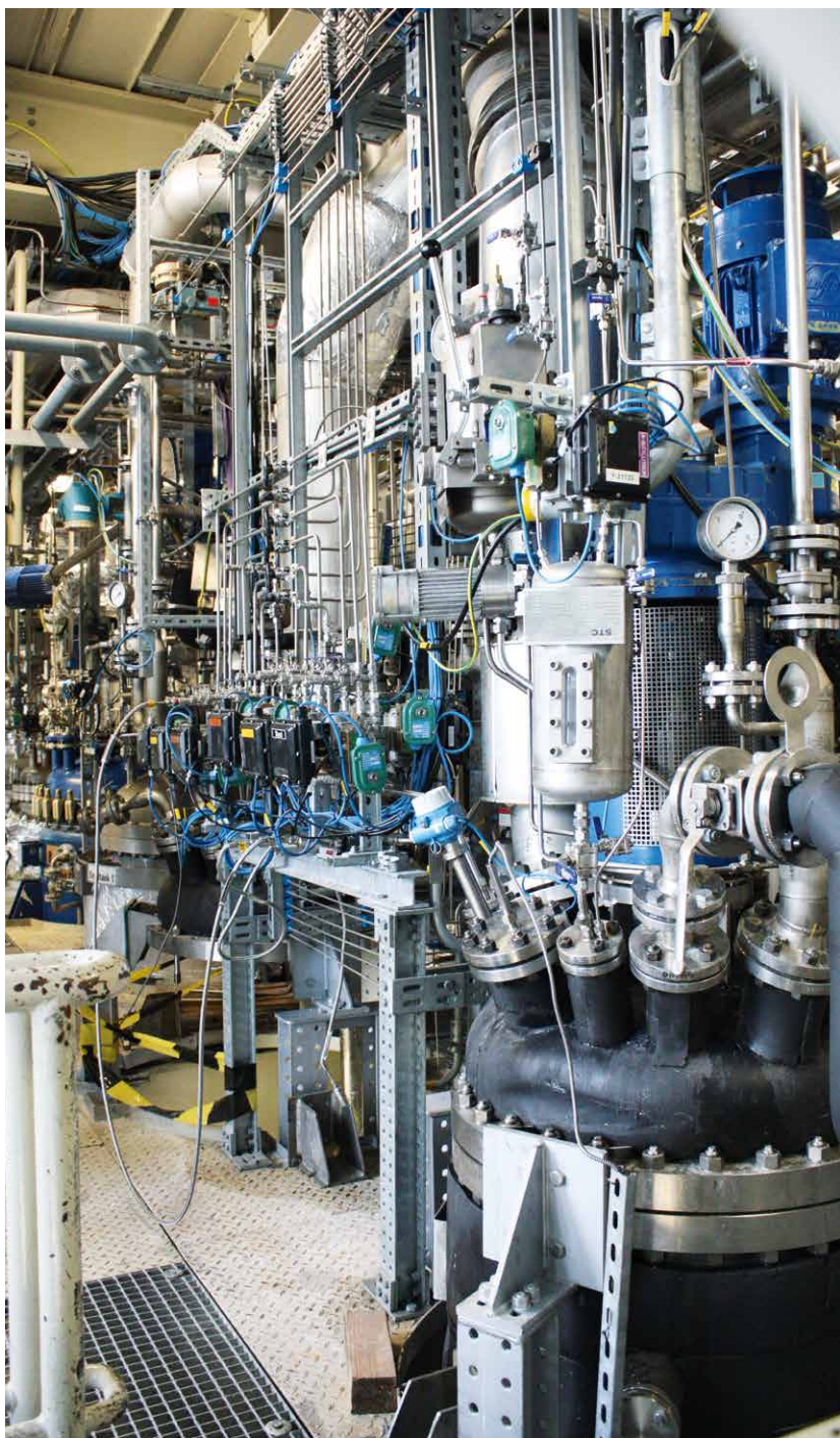
Rubber synthesis on a pilot scale (600 L reactor).
