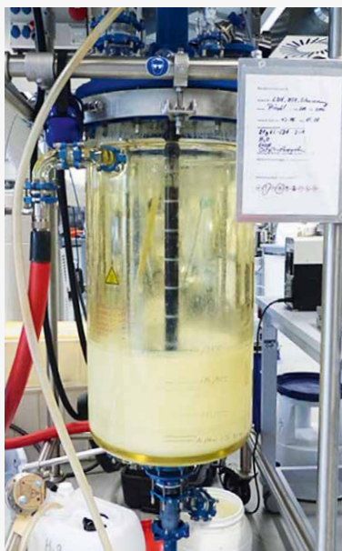
Scale-up equipment with 100 L batch reactor (left), semi-continuous centrifuge (center) and a pilot-scale spray dryer (right).
