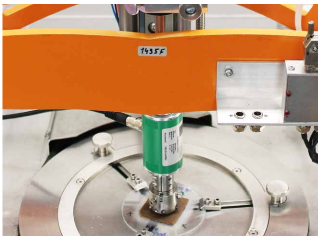
Figure 2 Tribometer for determining elastomer wear (above), ridge structure in the wear scar of an unreinforced elastomer (center), profile of a wear scar of a tire compound (below).
